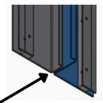
L-shape stops right door from being opened without an unlocked left door
