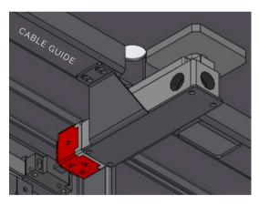
Access hole allows manual lock opening in case of electrical failure
